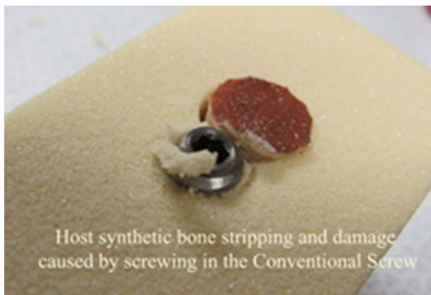
Fig. 6. Fixation with CIS screw causes some damage in the bone synthetic material. For the screw to drive forward a significant magnitude of torque is required resulting in high loads which strips some of the initial host threads.
